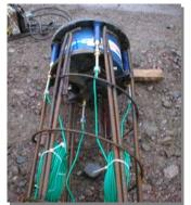
O-cell Assembly and Instrumentation.
